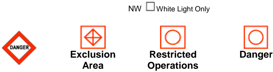
Figure 10 - Information and Regulatory Marks – When lighted may display any light rhythm not reserved for other types of aids.
